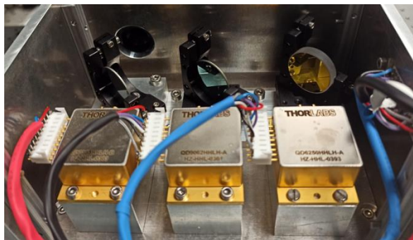
Fig. 1 Internal assembly of the three QCL mounted within the 3λ-QCL box.
