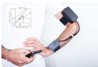
Fig. 1 Neogly, a novel device for non-invasive continuous glucose monitoring. The image shows the sensor connected to a portable battery and a handheld device with a user interface. Insert: Clarke Error Grid from data obtained with Neogly
